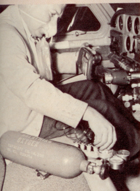
A portable oxygen unit offered by Puritan Compressed Gas Corporation for four-place aircraft consists of cylinder, manual regulator, quick-connect outlets, masks, rebreather bags and necessary tubing
