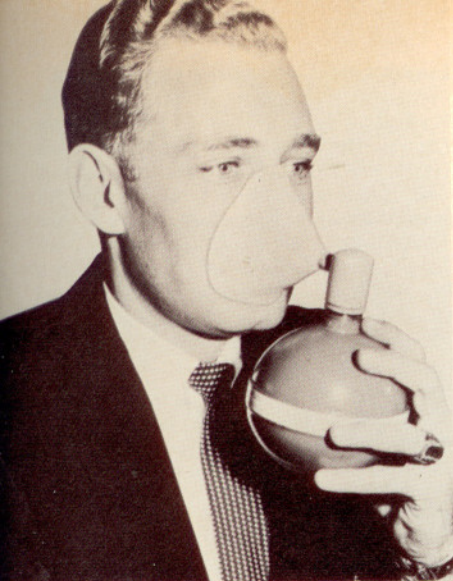
Emergency oxygen supply equipment for general aviation planes can be complex or as simple and economical as this Zep Aero portable "Zep-O-Life"
